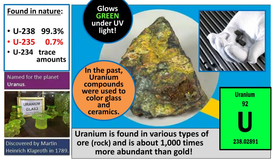
A single 7-gram pellet of *enriched* (processed to increase U-235 content to ~3-5%) Uranium produces as much energy as a ton of coal!
