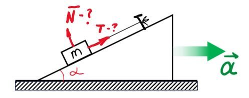
The frictionless wedge (see Figure above) is moving to the right with acceleration a. A brick of mass m is on the surface of the wedge and is attached with a thread as it is shown in the Figure. Find tension T of the thread and normal force N applied by the brick to the wedge.
