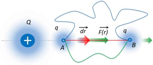
Figure 2. Potential energy difference between points A and B does not depend on the path geometry.
