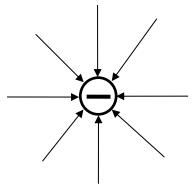
Figure 2. Electric field of a negative point charge.
