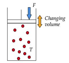
By changing this force we would change the pressure of the gas - the system will only come to equilibrium when forces acting on the piston are balanced. Finally, we could heat or cool the gas by bringing it to contact with hot or cold objects. We would assume that all gas has the same temperature at every moment of time (neglecting that the part closer to a heat source in reality heats faster). Temperature of the gas can be measured by a thermometer inside the container.
