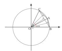
According to the definition given above, this must be equivalent to  $(a \cdot b) = ab \cos(\widehat{ab})$ , which could be straightforwardly verified from the drawings on the right.
