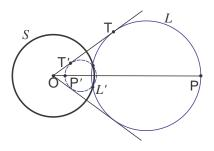
inversion image of the tangency point  $T \in L$  is the tangency point  $T' \in L'$  on the same tangent line.
