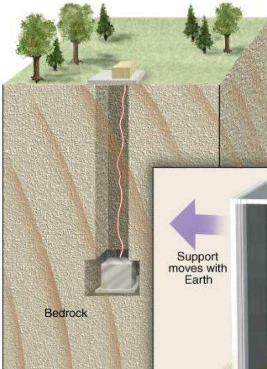
Different *seismograph* types are needed to record both vertical and horizontal ground motion:
